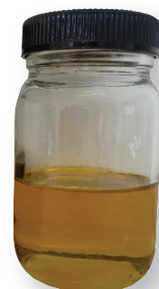
Transformer 8 with CJC™ Filter running 5 months
