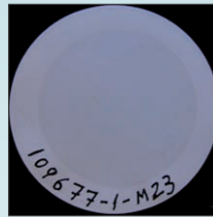
Millipore membrane AFTER filtration with the VRU, MPC <10
