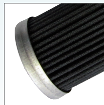
6 months WITH VRU: No varnish on the inline filter
