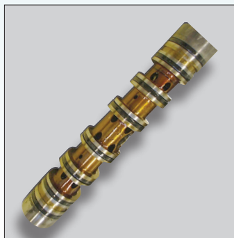
Varnish on valve spool
